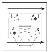
Slip the mounting bracket over the two screws and slide the bracket sideways until the screws heads capture the bracket.
