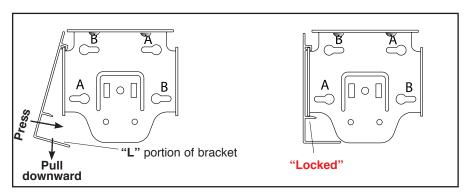
Attaching 4 inch Fascia Note: 4 inch fascia for use with SL-30 and SLG-400 requires notching.
