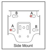
1.) Hold the mounting bracket in position in the window and mark the location where the screws should be positioned in either both A & A locations or B & B locations.
